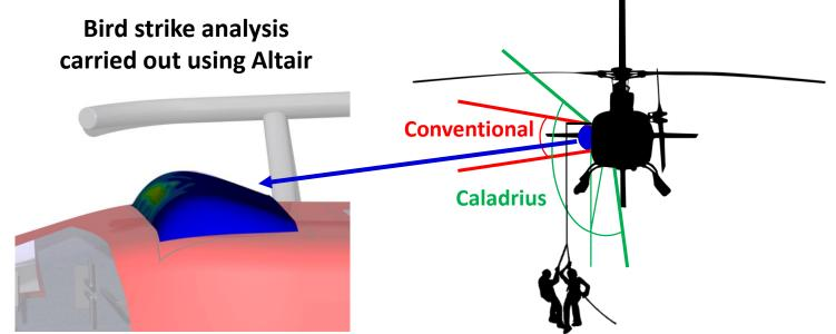
Bubble window geometry was designed after extensive aerodynamic studies for minimal impact in aircraft drag and increased lateral field of view
